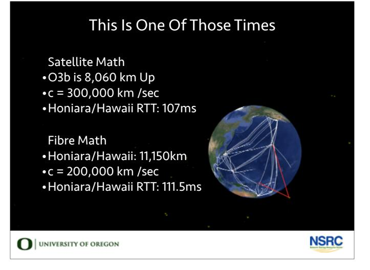
O3B is a constellation of satellites in medium earth orbit, each with ten 1.2gbps spot beams, covering earth from the equator plus or minus 45 degrees. Again via the What's Up database, you're seeing all of O3b's constellation in on the slide here, exactly as they were positioned when I took a screen shot a few days ago. There are a dozen up there now, and the constellation can accommodate up to 120. That's 1.4 Terabits of potential coverage.
