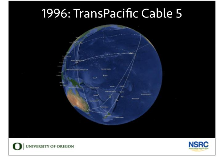
In 1996 TPC 5 lights up two pairs at 5gbps each in a loop connecting the US, Hawaii, Guam, and Japan. That's starting to sound like real capacity, at least for the 90s. Note Hawaii and Guam both starting to become important waypoints.
