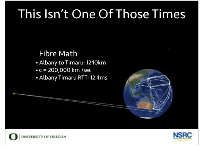
Note the speed of light inside glass is only 2/3 the speed of light in a vacuum.
