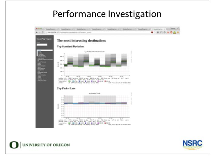
On the performance front, I spun up VMs around the world and pointed 360 probes at 45 Pacific networks. I was interested to see in general how telcos in the Pacific were performing latency-wise, and whether poor routing or peering practices might be hurting performance.
