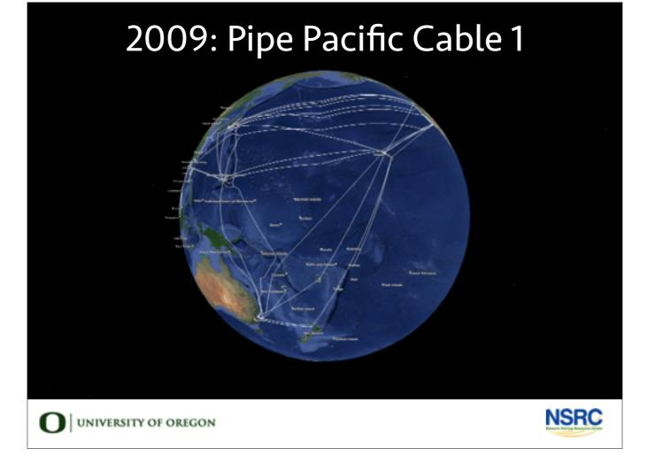
Rounding out 2009 we have Pipe's PPC1, which shot north to Guam (anyone surprised?) at 1.9 terabits per second with a branch to PNG, and potential for four more branches in between. Though the potential is there, the expense of taking the cable out of service for installation of a branch unit could be a deal breaker for anyone who wants to tap in. Branch units should really be installed before cables are commissioned.
