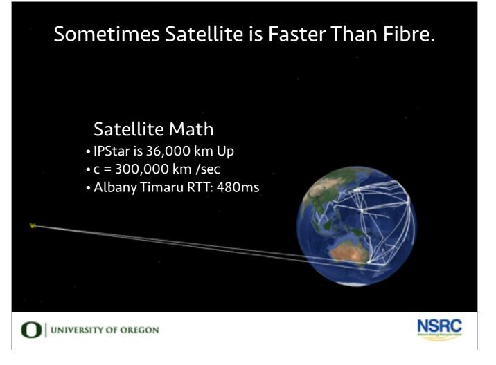
Let's do the math for IPStar, since most of us are familiar with it. By the way, this is a scale-accurate drawing of the path, if not the satellite itself.
