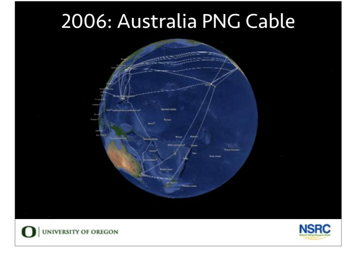
2006 has the cold, dead snake of PacRim West dragged off the seafloor and hauled to Port Moresby - recommissioned with a design bandwidth of just over a gigabit per second. From what I understand, regeneration in this cable is electronic, not optical, and E5 (565mbps) is as fast as electronic regeneration will work. So we've got two 565mbps bringing 1.1 gigabit per second into PNG.
