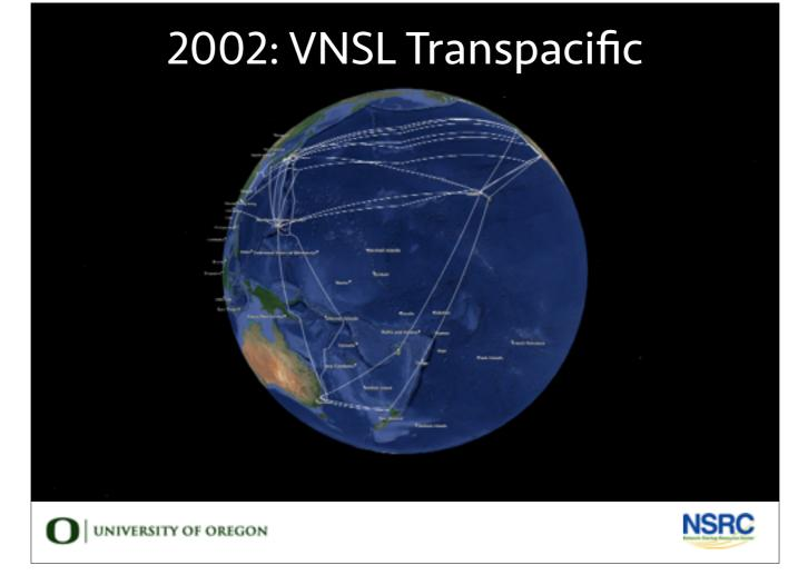
2002 brings the decommissioning of ANZCAN and the introduction of VNSL Transpacific (now known as TGN Pacific), nominally a US Japan cable, but with a branch down to Guam to meet the rest of the world there. Design capacity of 5 terabits per second. Heady days for fibre.
