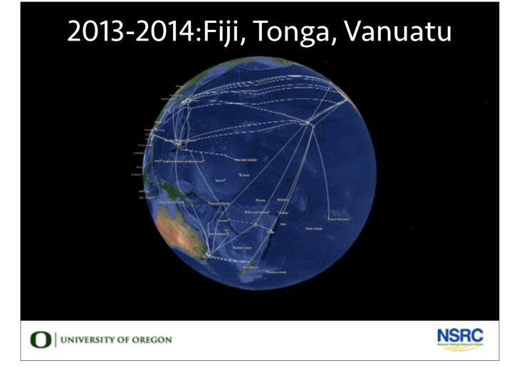
The last two years have seen two more small projects built by Alcatel Lucent Submarine Networks: the Tonga Suva cable in 2013, and the ICN cable from Vanuatu to Fiji in 2014. While both were lit at 20gbps, commercial arrangements are limiting use to the low hundreds of megabits on both.
